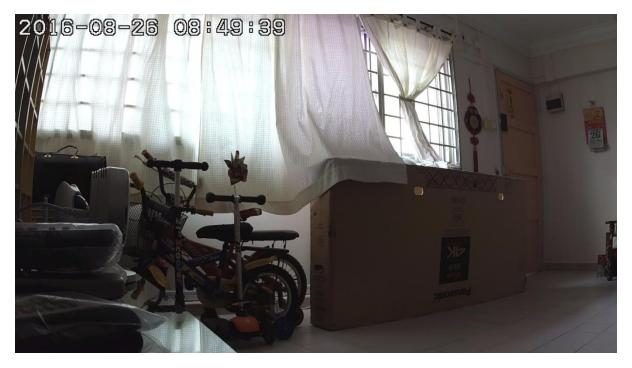
Image with WDR enabled. You can see now that the image that is against the light are adjusted so that you can see more in details, the bicycle area will show you more details in terms of the decals and wordings on it.
